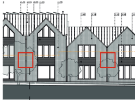
Fig. 1.1; Diagrammatic intention of a recessed downpipe in a brick cavity wall. Detail subject to construction method, U-value and rainwater calculations.
